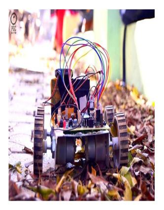
A Mobile Controlled Robot is a mobile device, which provides wide-range of wireless control ability to your robot unless your cell phone gets out of signal. The objective is to build a bot which can navigate using your instructions through DTMF controlled by your mobile phone and manoeuvre the bot through the arena.
