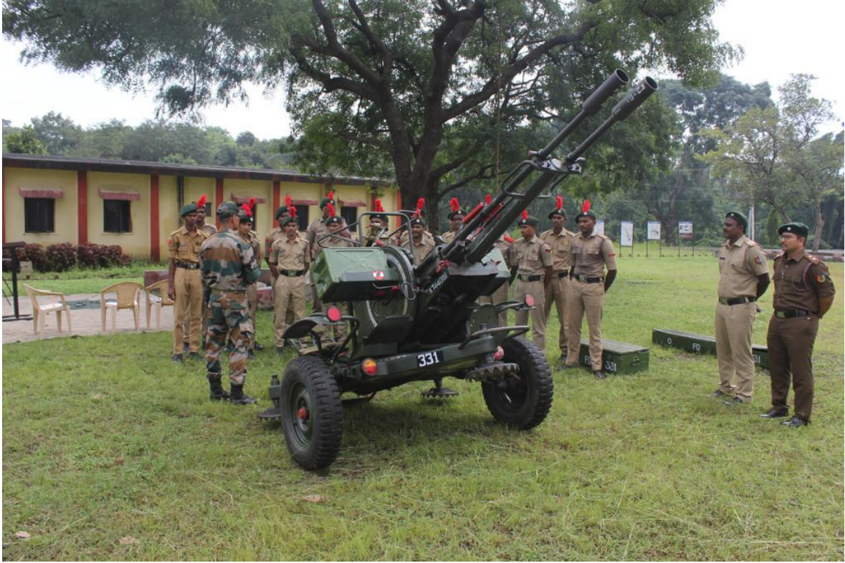
5. Cadets were briefed about the ZU-23-2 GUN, which aims at low-flying targets with a range of 2.5km.
